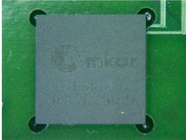
Figure 3. CSP Placed into Corner Dot Underfill.
